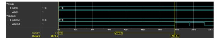
This figure shows a sample output and latency of the block when you specify a scalar input and set the **OFDM parameters source** parameter to Input port. In this example, the **FFTLen** port is set to 64, **CPLen** port is set to 16, **numLgSc** port is set to 6 and **numRgSc** port is set to 5, and **Maximum FFT length** parameter is set to 128.
