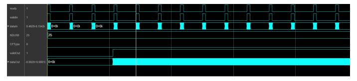
This figure shows the output data when you set the **Output data sample rate** parameter to Match output data sample rate to NDLRB parameter. For NDLRB value 25, the output sample rate is 7.68 MHz, and the block returns valid output data at every fourth cycle.
