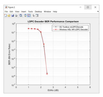
This plot shows the performance of the block for a 4-bit LLR input when you set the  ${\bf Algorithm}$  parameter to Normalized min-sum .
