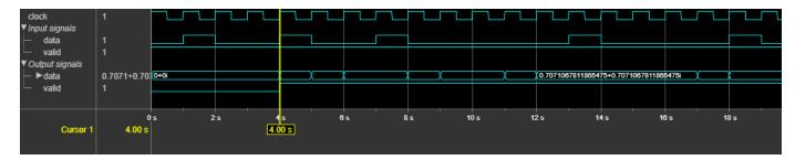
This figure shows a sample output when you select BPSK, QPSK, 16-QAM, 64-QAM, 256-QAM, and pi/2-BPSK modulations by using the **modSel** input port. The latency of the block varies with the modulation selection.
