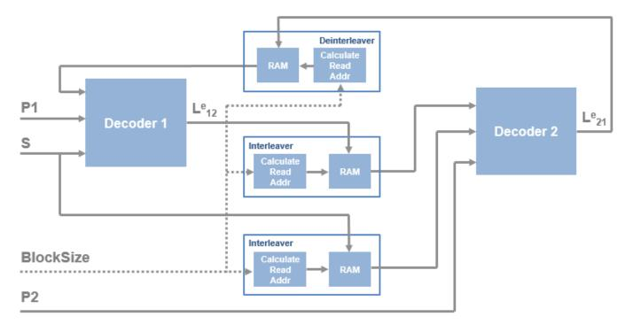
output is routed back to the input for the next half-iteration. The interleaver computes the interleave indexes from the block size. For details of the interleaver implementation, see LTE Turbo Encoder.
