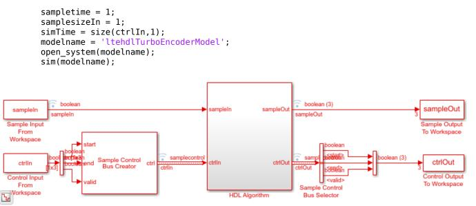
The Simulink model exports sampleOut\_ts and ctrlOut\_ts back to the MATLAB workspace. Deserialize the output samples, and compare the framed data to the reference encoded frames.
