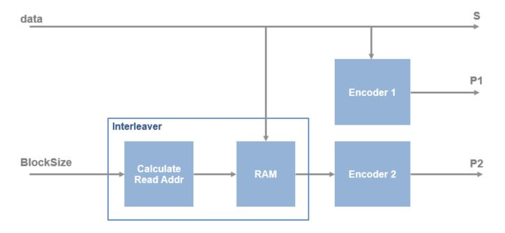
When **Block size source** is set to **Property**, the block uses two constant coefficients to derive the read addresses for the fixed block size. When **Block size source** is set to **Input port**, the algorithm saves the 188 pairs of coefficients in a ROM (< 5 Kb). Then the block reads the matching pair at run time to derive the interleave memory read addresses.
