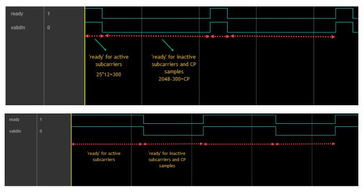
These figures show the timing diagrams of the **ready** output signal for NDLRB values 25 and 100, respectively.
