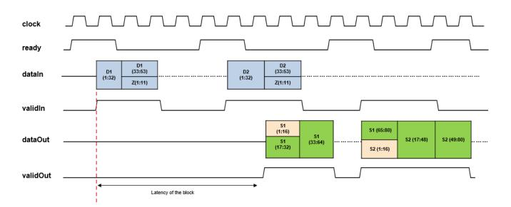
To provide 53 active data subcarriers of vector length 32, two cycles are needed. In this case, you must send the first set of data samples as D1(1:32), send the second set of data samples as D1(33:53), and pad the remaining samples with zeros Z(1:11) to make the complete vector. Similarly, the block processes D2 based on the block parameter values.
