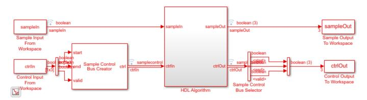
The Simulink model exports sampleOut\_ts and ctrlOut\_ts back to the MATLAB workspace. Deserialize the output samples, and compare the framed data to the reference encoded frames.
