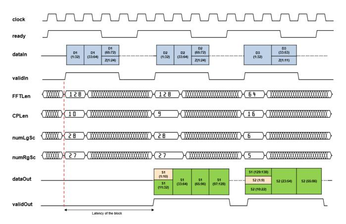
To provide 73 active data subcarriers of vector length 32, three cycles are needed. In this case, you must send the first set of data samples as D1(1:32), send the second set of data samples as D1(65:96), send the third set of data samples as D1(65:72), and pad the remaining samples with zeros Z(1:24) to make the complete vector. Similarly, the block processes D2 based on the port values.
