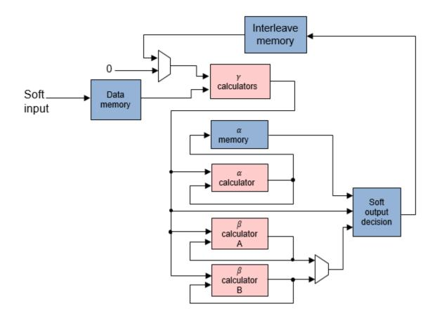
In a normal BCJR architecture, the algorithm cannot compute β until the entire frame is in memory. It must perform a full-frame forward trace and then a full-frame backward trace, which means the latency of one half-iteration is two frame lengths. The required memory is *BlockSize\*NumStates\*DataWidth*. In this case, *NumStates* is eight, from LTE standard TS 36.212 [1].
