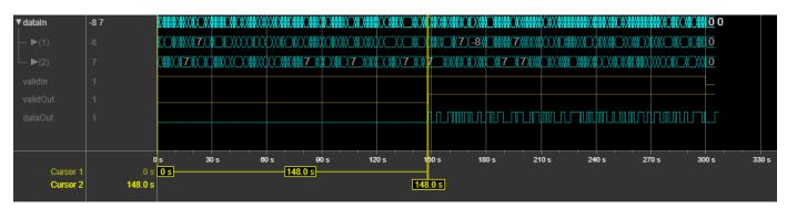
The second waveform shows three frames in terminated operation mode. The input is unsigned 4-bit samples, and the block is using the trellis (7,[171 133 112]). The **Traceback depth** is 32. The input and output **ctrl** buses are expanded to show their three control signals. The latency from each input **ctrl.start** to output **ctrl.start** is also 148 clock cycles.
