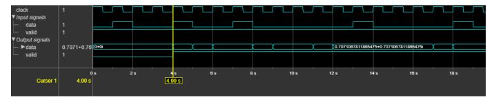
This figure shows a sample output when you select BPSK, QPSK, 16-QAM, 64-QAM, and 256-QAM modulations by using the **modSel** input port. The latency of the block varies with the modulation selection.
