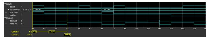
• Frame mode — When the puncture vector element is 1, the block stores the corresponding input data in a buffer. It waits till it encounters the next 1 in the puncture vector and then provides the previous buffered data as output.
