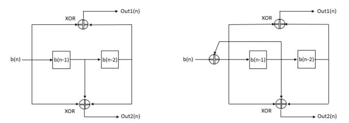
b(n) represents input data bit stream and b(n-1) and b(n-2) represent the 2-bit shift register of the encoder. *Out1(n)* and *Out2(n)* represent the 2-bit output. From this figure, you can calculate the block mask parameters based on the Convolutional codes concepts. For more information about
