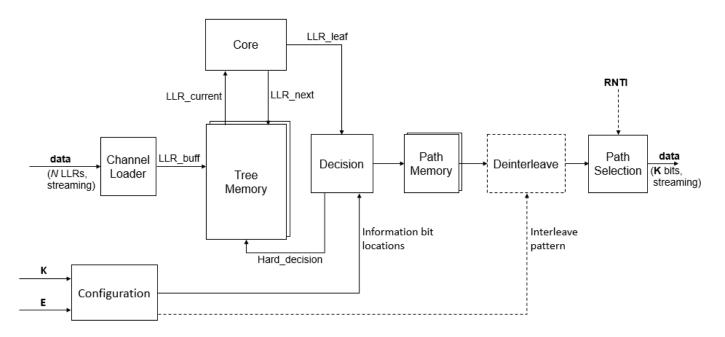
The block uses the Configuration stage when the **K** and **E** input port values change. The block computes the locations of the information bits and passes them to the Decision stage. Because the mapping patterns are computed as needed, rather than stored in hardware, the block supports all **K** and **E** values within the supported range. The Configuration stage also computes the interleave pattern when you set the **Link direction** parameter to Downlink.
