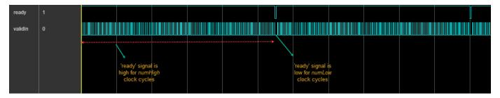
numHigh = (FFT length + CP length -1) \* Maximum FFT length / FFT length + 1 = (128 +10 -1) \* 16 + 1 = 2193 clock cycles.
