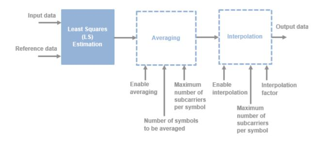
The Averaging block accepts the LS estimates and averages the corresponding subcarriers with valid LS estimates over the number of OFDM symbols to be averaged provided in the block mask. This figure shows a sample output of the OFDM Channel Estimator block when only averaging is enabled. In this case, the **Number of symbols to be averaged** parameter is set to 4, **Maximum number of subcarriers per symbol** parameter is set to 16, and the **numScPerSym** port is set to 4.
