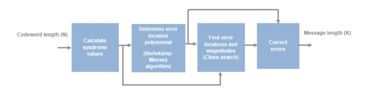
This block uses the Berlekamp-Massey decoding algorithm. For information about this algorithm, see "Algorithms for BCH and RS Errors-only Decoding".
