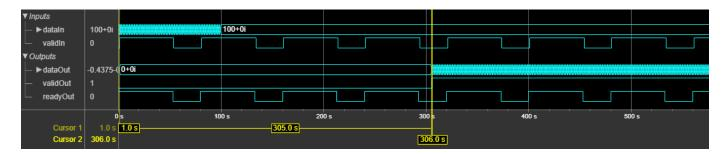
This figure shows a sample output and latency of the block when you specify a scalar input and set the **OFDM parameters source** parameter to Input port. For this example, **FFTLen** is set to 64, **CPLen** is set to 16, **Insert DC null status** is set to on, **numLgSc** and **numRgSc** are set to 6 and 5, respectively, and **Maximum FFT length** is set to 128.
